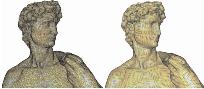
Figure 2: Nonuniform mesh ( left ) and its uniform counterpart after uniform remeshing ( right ). [All+08]
